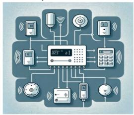
No device is connected to a LAN, WAN, or the internet. However, wireless devices connected to the alarm panel in the picture above are not connected to the internet. Firmware updates are allowed via the USB port on the alarm panel if it or any of its devices do not connect to a LAN, WAN, or the internet. In this case, it is not in the scope of the PSTI Act.
